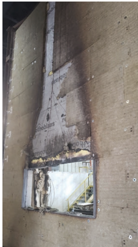
FIGURE 9: Test 1 completed – Window burner extinguished with ongoing flaming within test room (left); damage to assembly layers with mineral wool manually removed (right)
