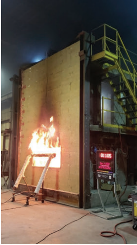
FIGURE 8: Test 1 underway (left); flames impinging on mineral wool above window (right)
