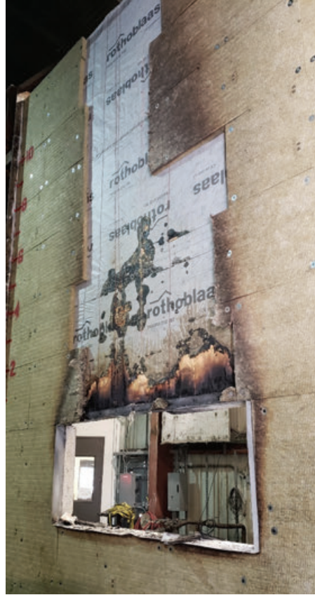
FIGURE 10: Test 2 underway – Flames extending above window (left); post-test showing damage to layers after mineral wool manually removed (right)
