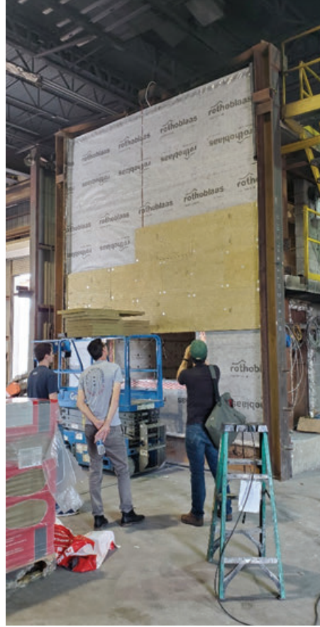
FIGURE 4: Test 1 setup – Installation of WRB (left); installation of mineral wool insulation (right)
