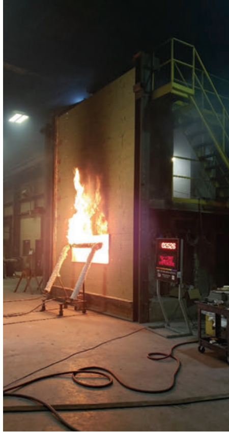
FIGURE 10: Test 2 underway – Flames extending above window (left); post-test showing damage to layers after mineral wool manually removed (right)
