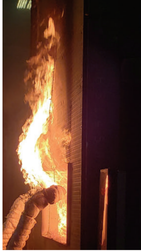
FIGURE 8: Test 1 underway (left); flames impinging on mineral wool above window (right)
