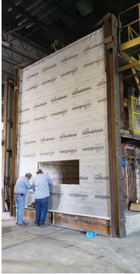
FIGURE 4: Test 1 setup – Installation of WRB (left); installation of mineral wool insulation (right)
