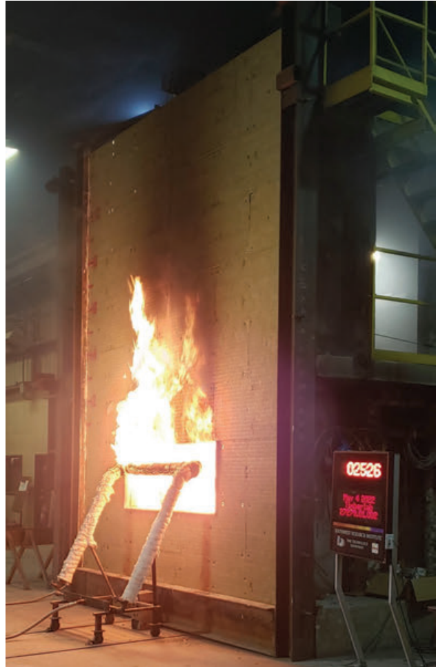
FIGURE 1: NFPA 285 test showing exterior burner in position
