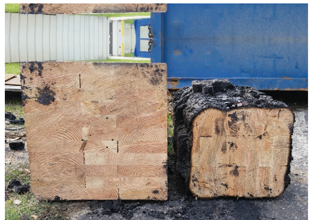
Glulam column before and after 2-hour fire test
