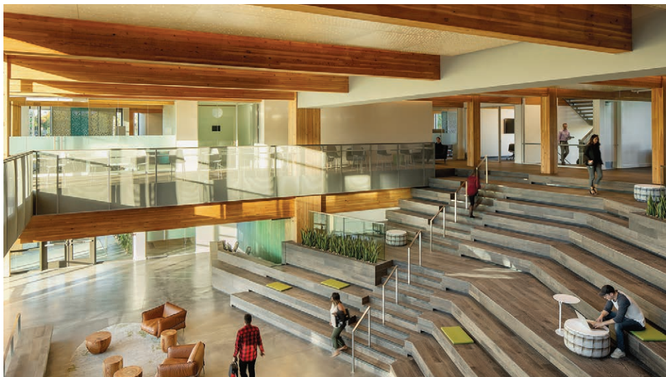
First Tech Federal Credit Union / Hillsboro, Oregon / Hacker / Kramer Gehlen & Associates / Swinerton Five-story, Type III-B office building with a hybrid mass timber and steel structural system
