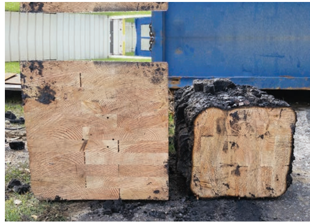
Partially charred glulam column pre (left image) and post (right image) 2-hour fire test
