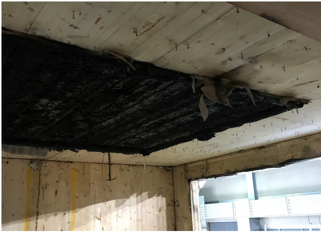
Figure 10: Charred CLT post fire during the ATF lab tests
