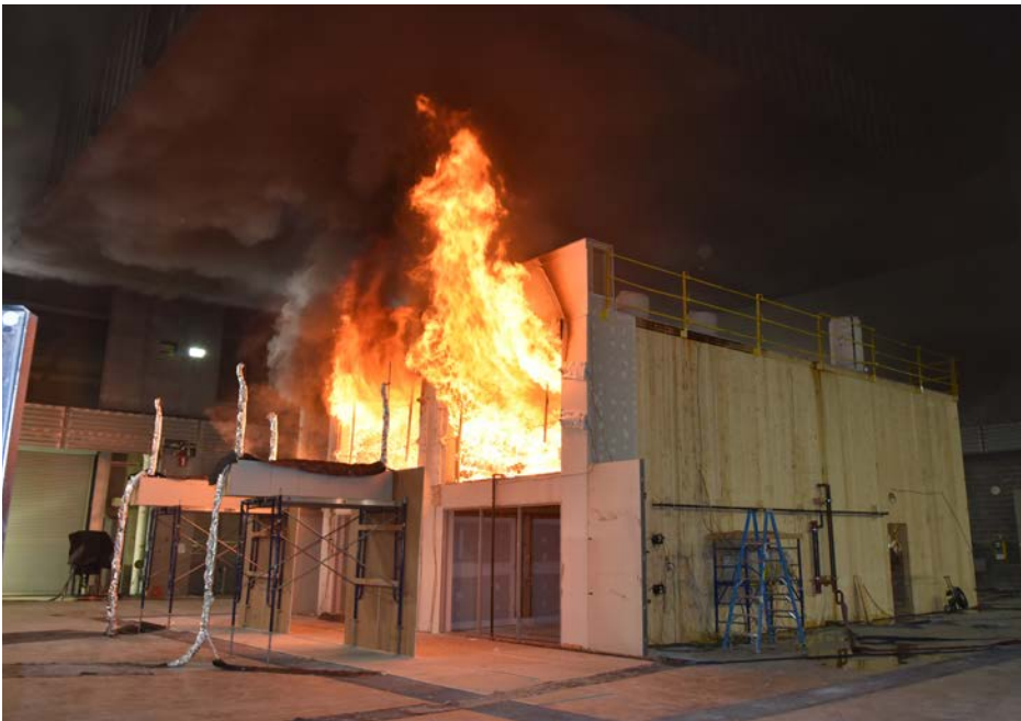
Figure 3: Mass timber compartment fire testing at ATF lab
