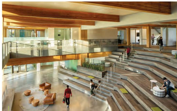
According to Swinerton, using CLT and glulam instead of steel for the First Tech Federal Credit Union's new campus resulted in a 4 percent cost savings and four fewer months of construction. (See cover photo.)
