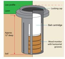
Termite bait systems require ongoing contracts with a pest management professional. If baits are chosen as the only method of treatment, there is nothing protecting the structure should the building owner discontinue the maintenance contract.
