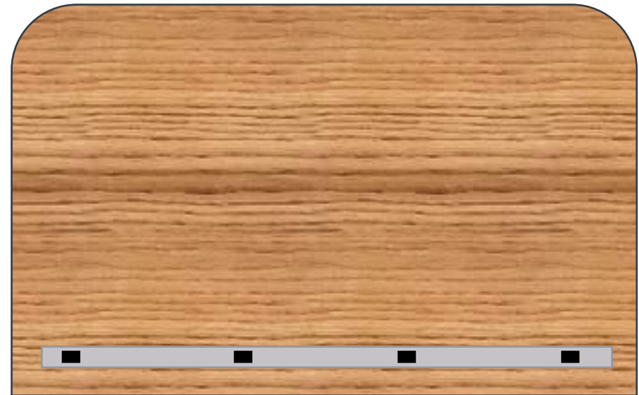
Grill Installed at Balcony Ceiling with Perforations Greater 1/150 of Balcony Deck Surface Area
