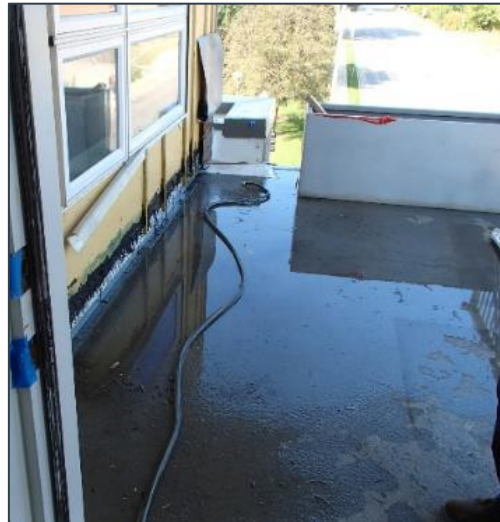
Water testing to determine possible areas of water intrusion at deck to wall transition - WPM
