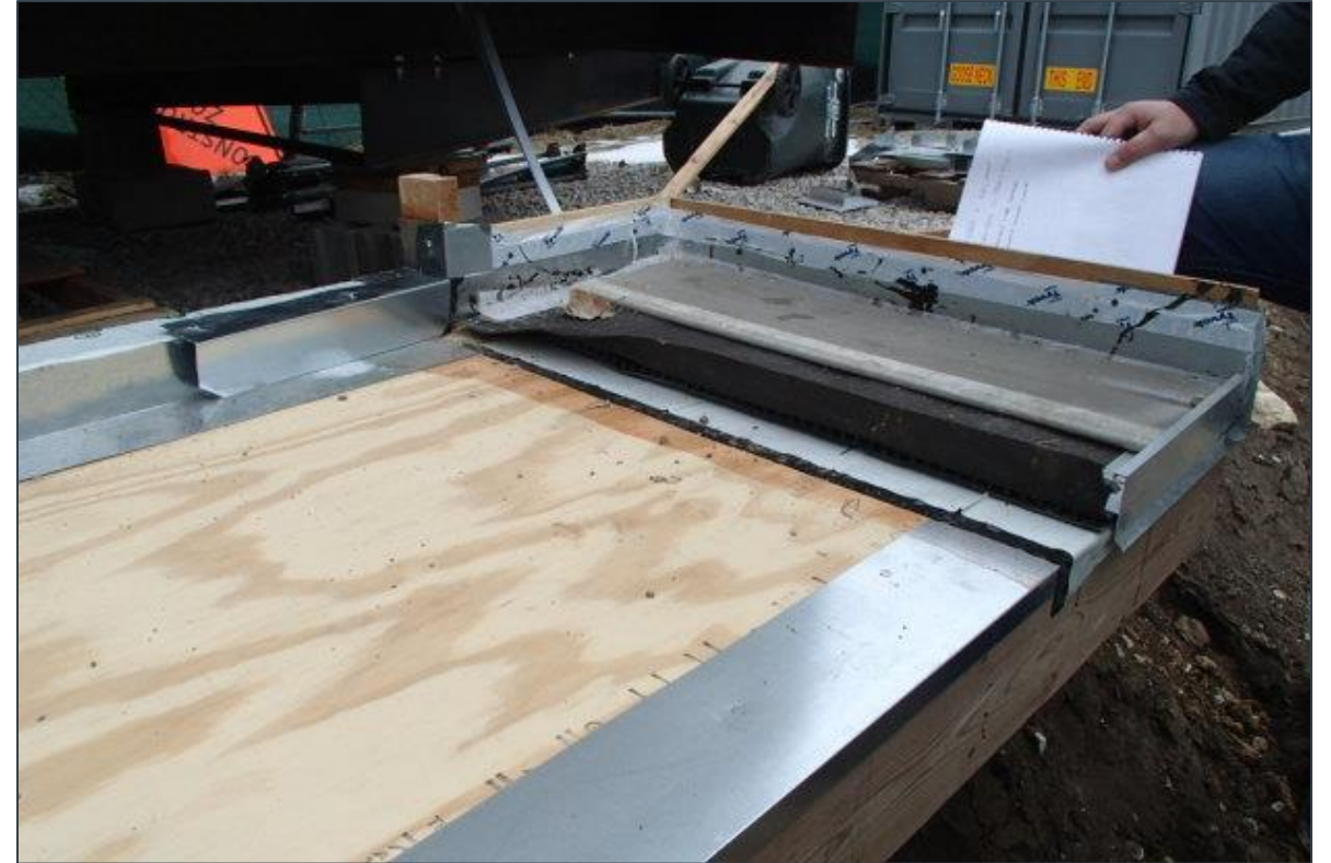
Pre-construction testing and inspection of deck waterproofing system field mockup - WPM
