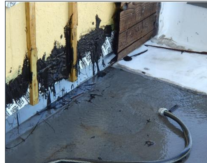
Water testing to determine possible areas of water intrusion at deck to wall transition - WPM
