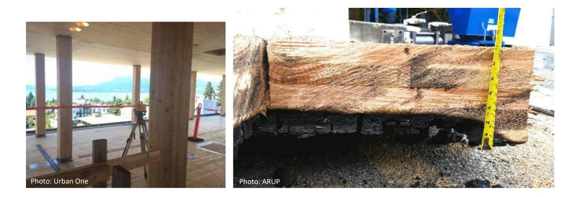
In tall buildings, preventing fire re-growth is key. Fire re-growth is a phenomenon in which the heat-release rate of a fire intensifies following a decay phase. Fire re-growth can be initiated when delamination occurs, as this exposes un-charred wood surfaces, thereby resulting in an influx of fuel available for consumption by the fire.
