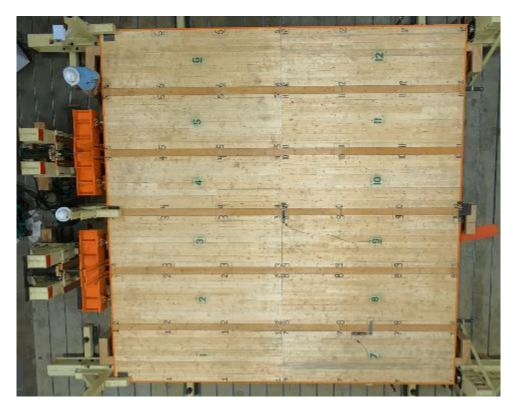
Photo: CLT Diaphragm Testing, Credit: AWC
