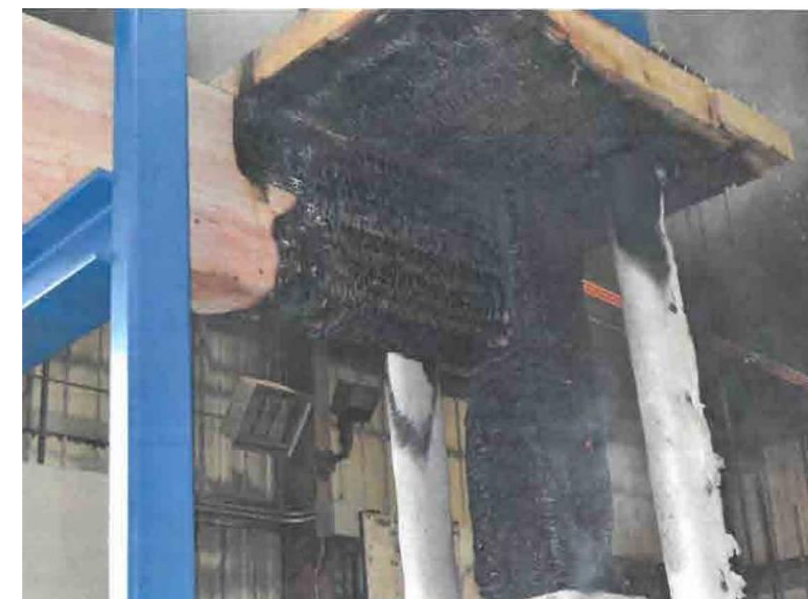
Example fire test of a beam to column connection (MTC Solutions)
