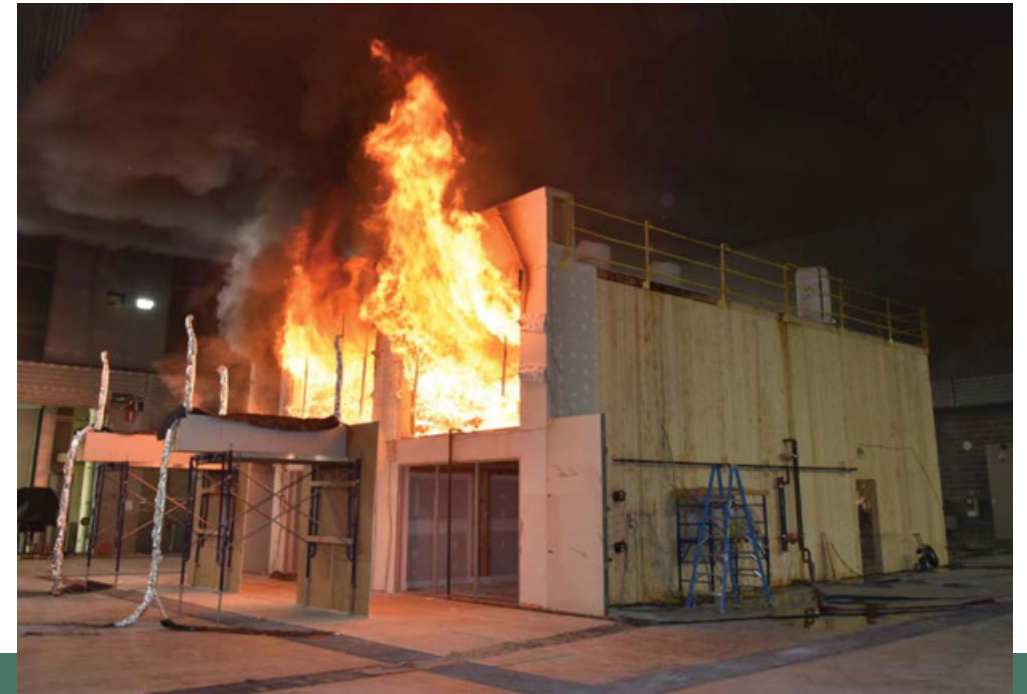
Mass Timber Fire Testing at ATF Lab (2017)
