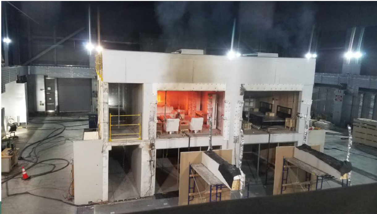
Mass Timber Fire Testing at ATF Lab (2017)
