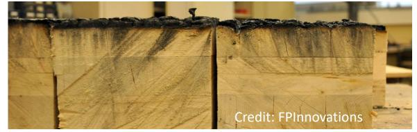
Nominal char rate of 1.5"/HR is recognized in NDS. Effective char depth calculated to account for duration, structural reduction in heat-affected zone
