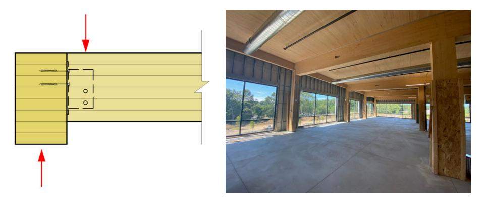
Connection FRR and beam reactions could impact required beam/column sizes
