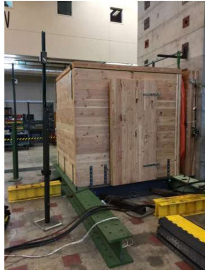
Fig 19 Safe room tied down to strong floor
