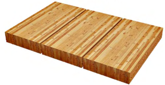
Glue-Laminated Timber (GLT) Plank orientation
