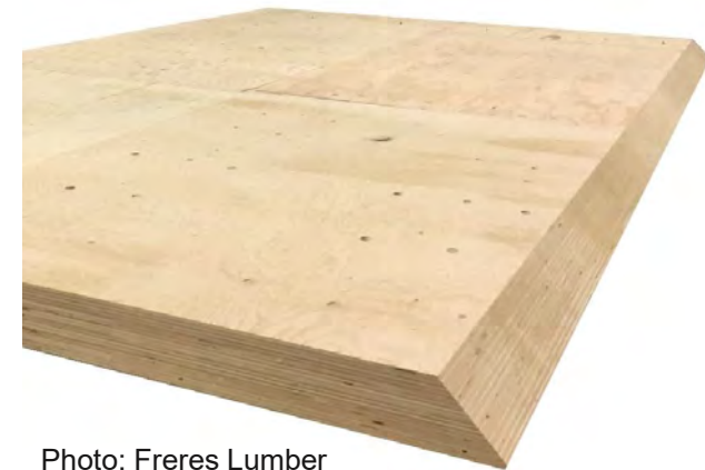
Cross-Laminated Timber (CLT) SCL laminations
