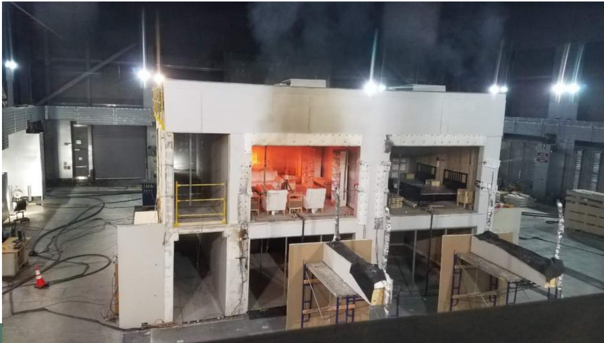
Mass Timber Fire Testing at ATF Lab (2017)
