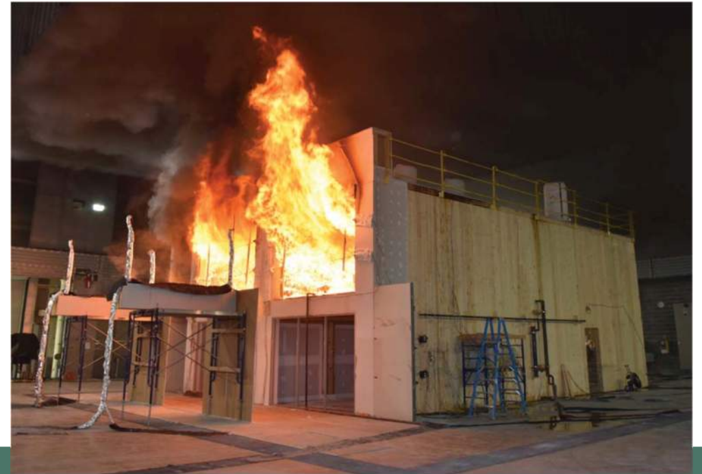
Mass Timber Fire Testing at ATF Lab (2017)
