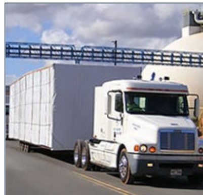
Modules Are Transported to the Construction Site
