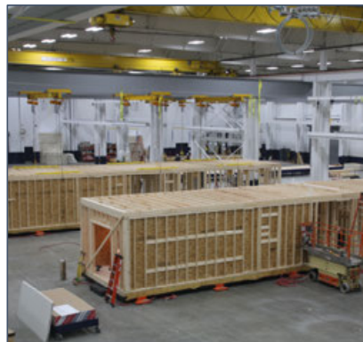
Modular Units are Manufactured Inside Climate Controlled Factory
