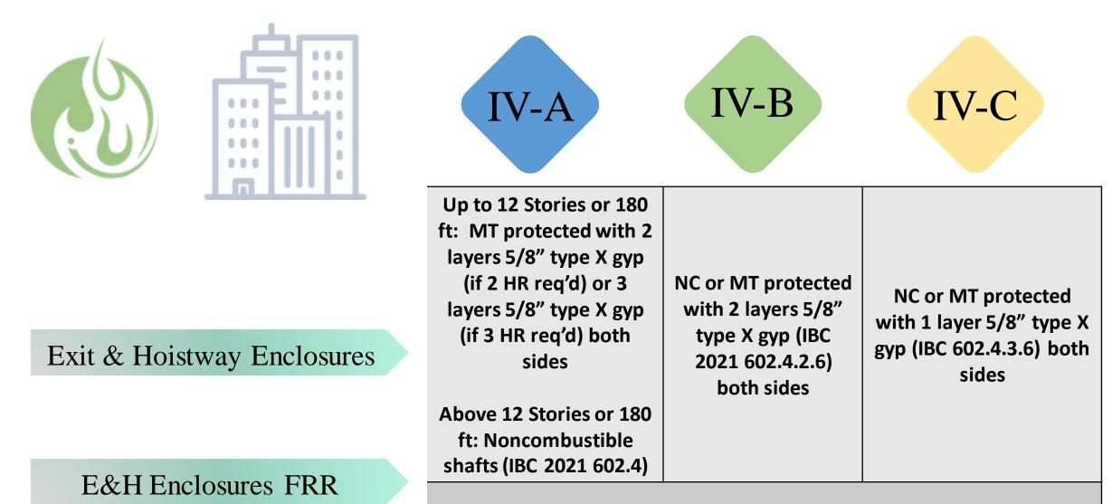
2 HR (not less than FRR of floor assembly penetrated, IBC 713.4)
