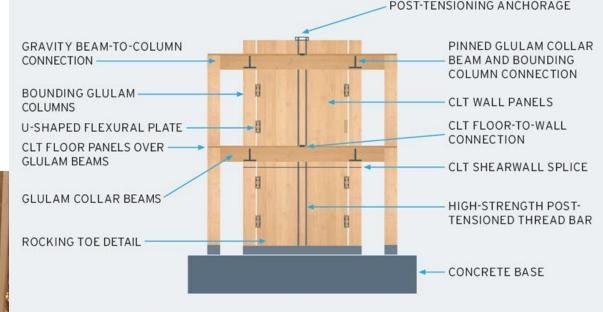
ELEVATION - POST-TENSIONED ROCKING WALL (STATIC STATE)
