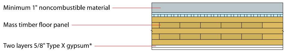
\*Applicable to most locations; limited exposed mass timber permitted in IV-B
