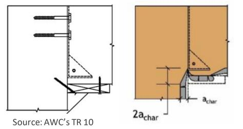
2. Engineering analysis that demonstrates that the temperature rise at any portion of the connection is limited to an average temperature rise of 250° F (139° C), and a maximum temperature rise of 325° F (181° C), for a time corresponding to the required fire resistance rating of the structural element being connected. For the purposes of this analysis, the connection includes connectors, fasteners, and portions of wood members included in the structural design of the connection.
