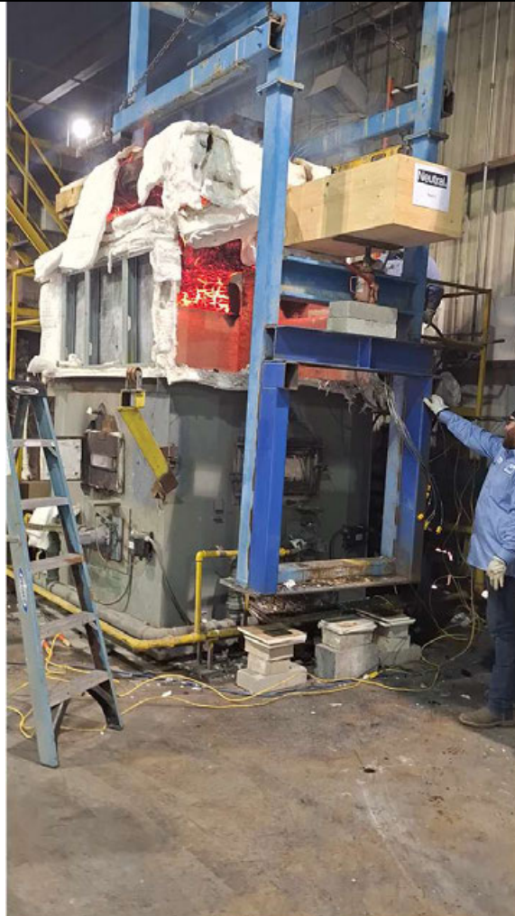
Glulam beam to column fire resistance test to ASTM E119 – removal of assembly from furnace
