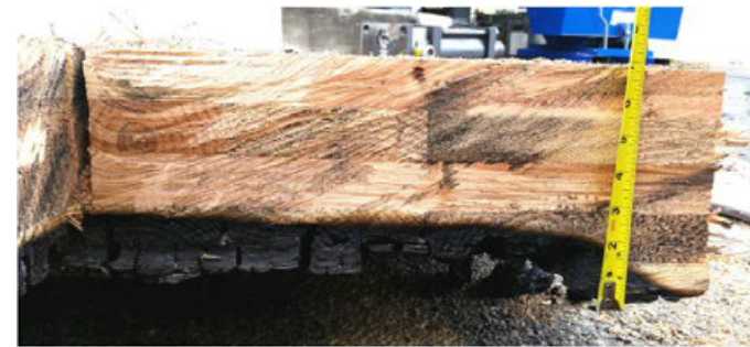
5 ply CLT after 2 hrs fire test
