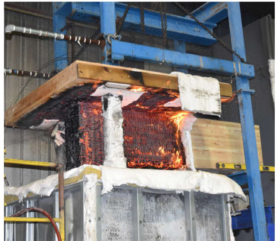
Glulam beam to column assembly fire test, FRR 2 hrs
