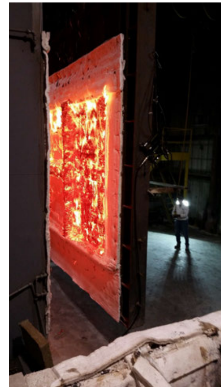
CLT wall after 2 hrs fire test
