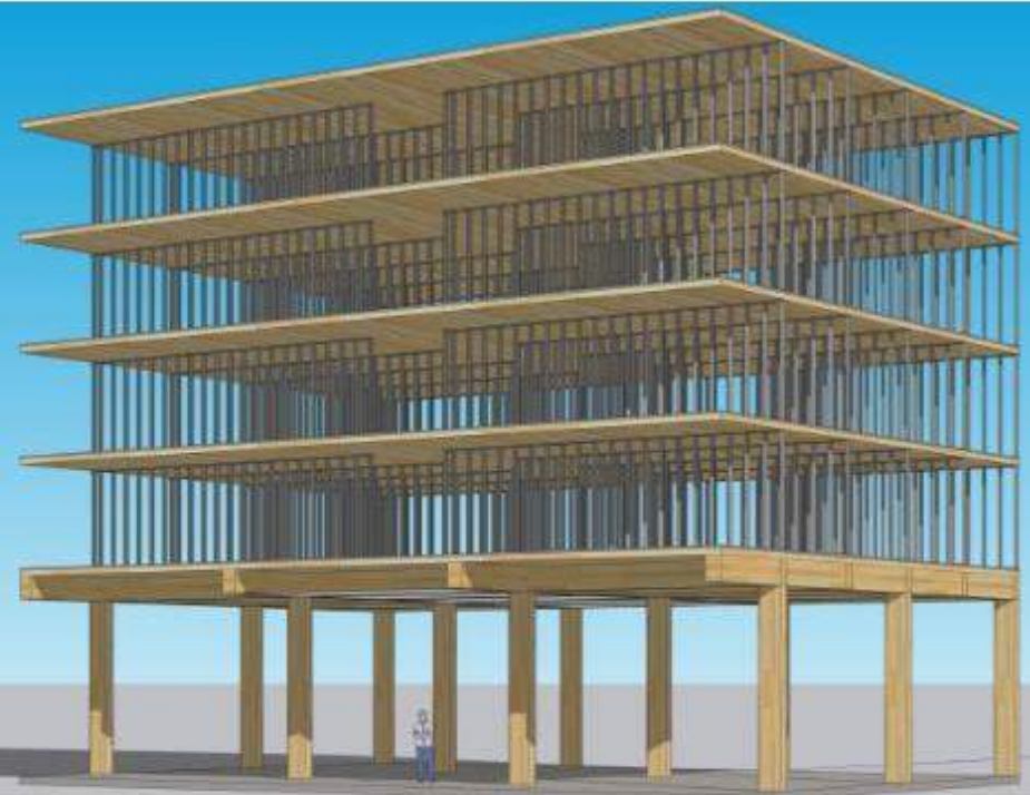
Timber Scheme 2: steel stud with timber deck on glu-lam post and beam podium
