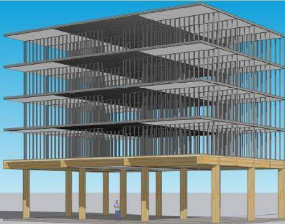
Timber Scheme 1: steel stud and deck on glu-lam post and beam podium
