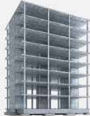
Reference 2 Concrete Flat Slab; Concrete Cores
