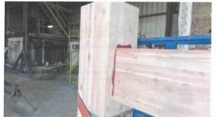
Figure A-4. Column and Beam Connection.
