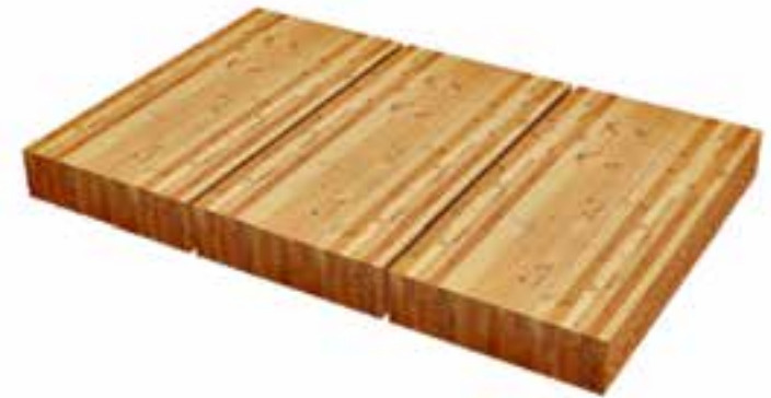
Glue-Laminated Timber (GLT) Plank orientation
