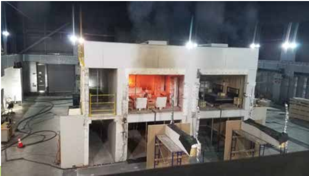
Mass Timber Fire Testing at ATF Lab (2017)
