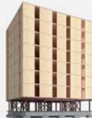
Timber Use 4 Timber Floors & Shear Walls; Steel Frame Podium
