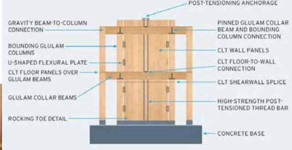
ELEVATION - POST-TENSIONED ROCKING WALL (STATIC STATE)
