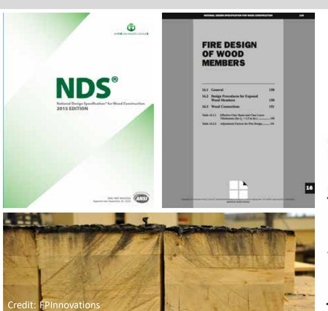
NDS Chapter 16 includes calculation of fire resistance of NLT, CLT, Glulam, Solid Sawn and SCL wood products
