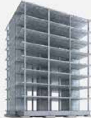
Reference 2 Concrete Flat Slab; Concrete Cores
