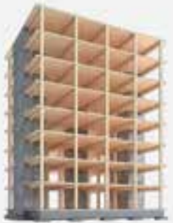
Timber Use 2 Timber Post, Beam, & Plate; Concrete Cores
