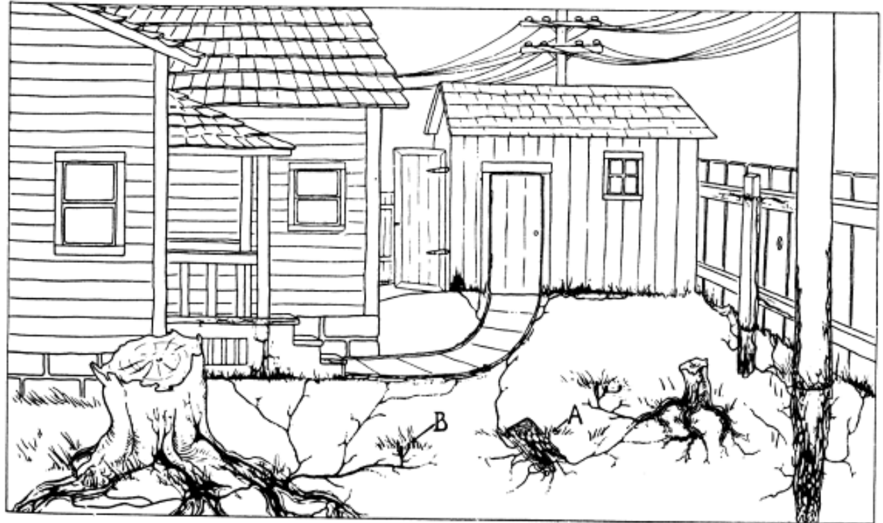
Fig. 50. This sketch combines the sorts of conditions found to prevail in many localities where wood has been improperly used. Unprotected wood in or on the ground makes possible both settlement and rapid increase of the subterranean termites. Workings in stumps, poles, posts, sidewalks, and wood of buildings are shown in black, as are the galleries within the earth. A marks the supposed original point of entry of one of the colonizing pairs, and B the points of emergence of swarming alates at the proper season.
