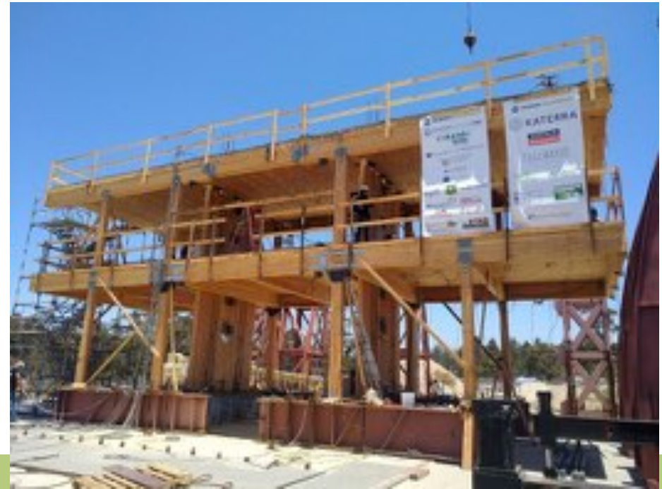
Mass Timber Shake Table Test at UCSD
