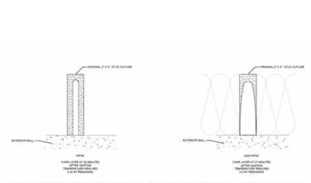
Figure 5: FRTW and Non-FRTW Stud Walls at 70 Minutes After Fire Exposure of Gypsum Board Wall Point of FRTW Wall Failure
