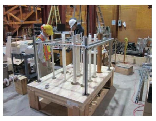
Most firestopping systems include combination of fire safing (eg. noncombustible materials such as mineral wool insulation) plus fire caulk
