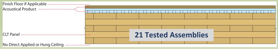
Table 3: CLT Floor Assemblies without Concrete/Gypsum Topping, with Wood Sleepers, Ceiling Side Exposed
