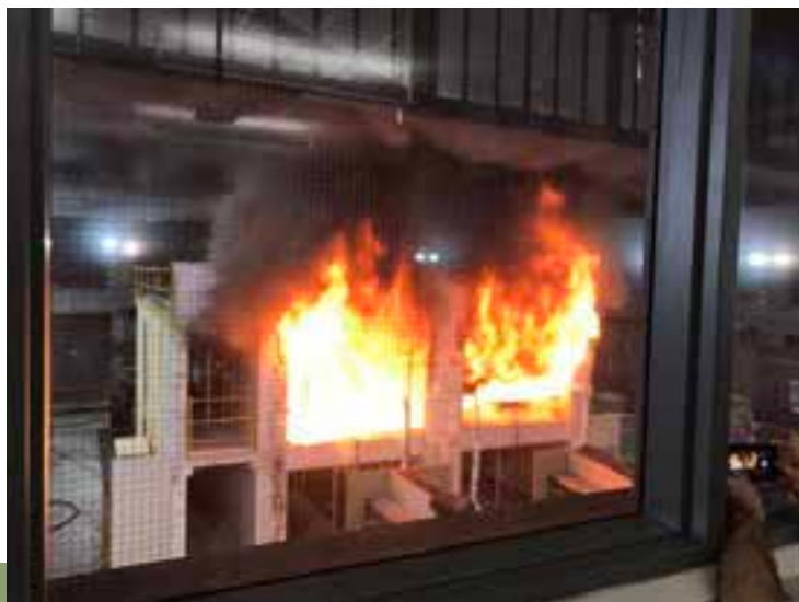
Mass Timber Fire Testing at ATF Lab
