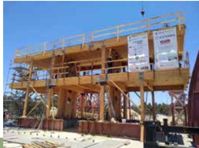
Mass Timber Shake Table Test at UCSD
