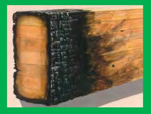
2015 NDS CHAPTER 16 INCLUDES CALCULATION OF FIRE RESISTANCE OF NLT, CLT, GLULAM, SOLID SAWN AND SCL WOOD PRODUCTS
