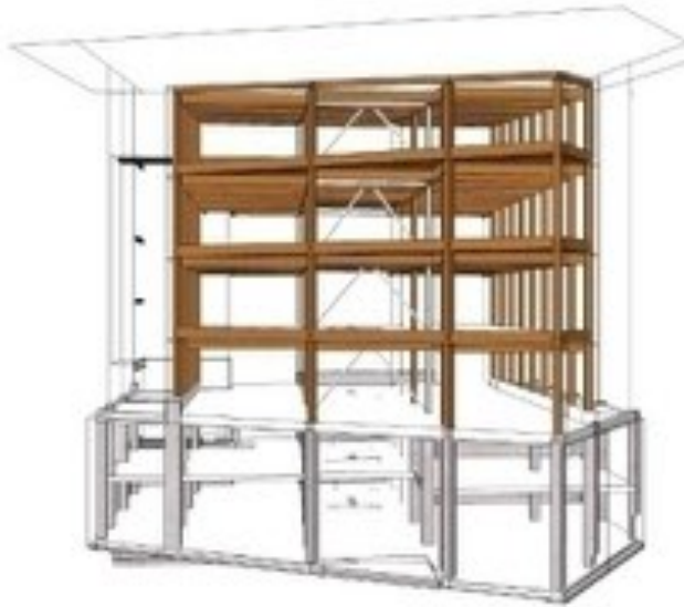
250 YEAR STRUCTURE HEAVY TIMBER, CONCRETE & STEEL
