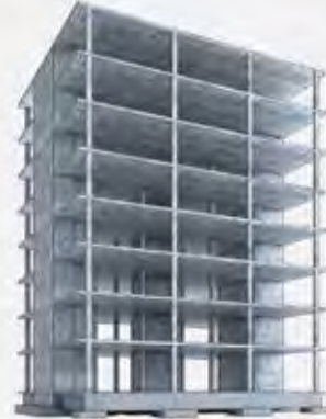
Reference 2 Concrete Flat Slab; Concrete Cores
