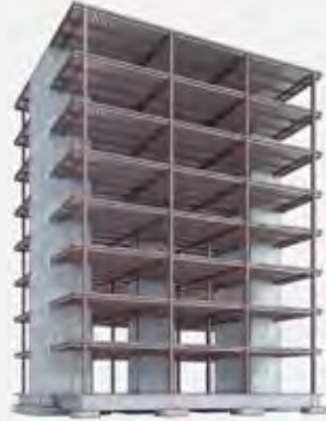
Reference 1 Concrete Slabs on Steel Deck; Steel Frame; Concrete Cores
