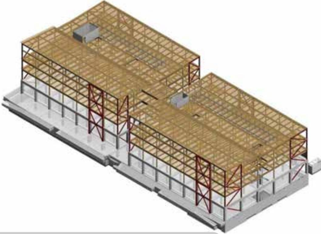
Buckling Restrained Braced Frame (6 per wing)
