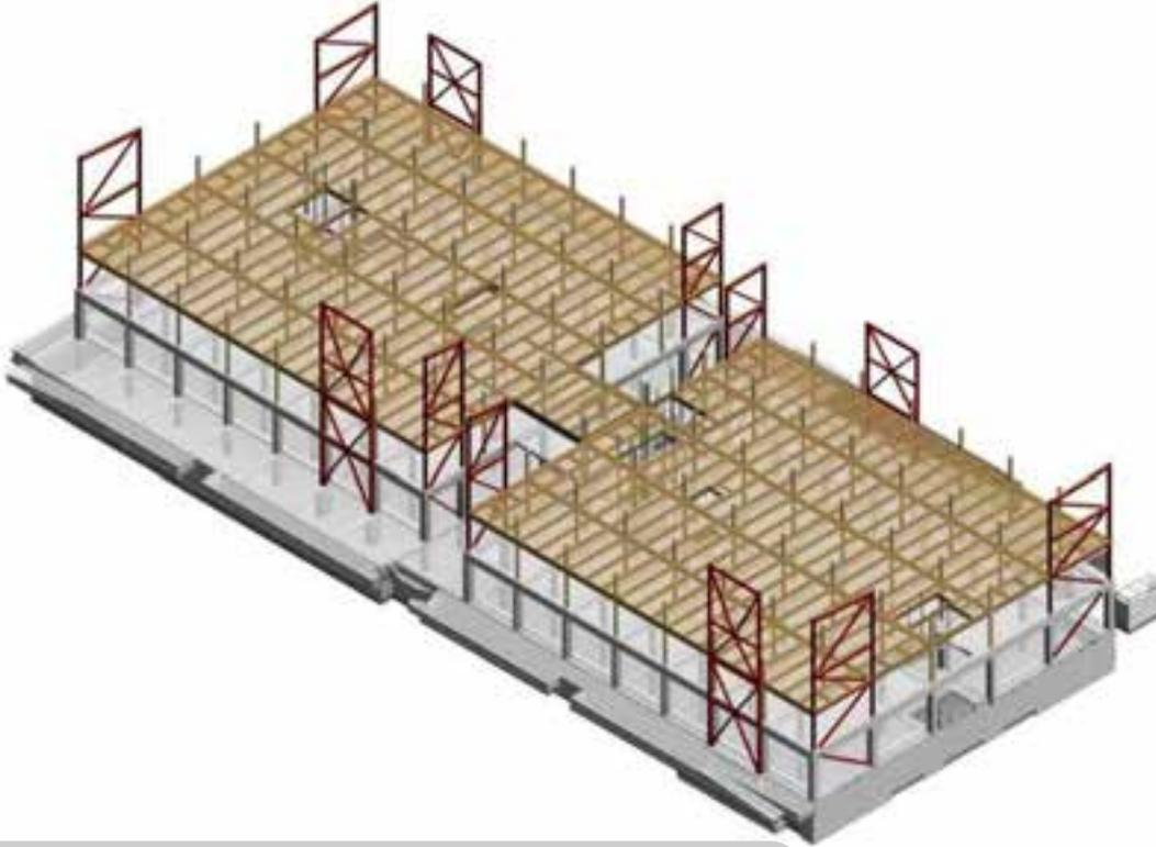
Buckling Restrained Braced Frame (6 per wing)
