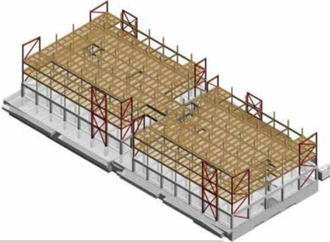
Buckling Restrained Braced Frame (6 per wing)
