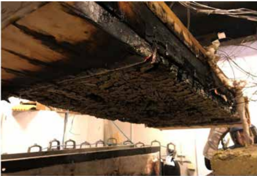
Fire Safety Challenges of Tall Wood Buildings – Phase 2: Task 5 – Experimental Study of Delamination of Cross Laminated (CLT) Timber in Fire
