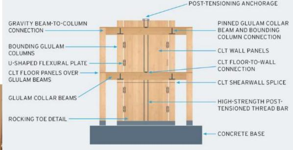
ELEVATION - POST-TENSIONED ROCKING WALL (STATIC STATE)
