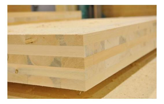
Concrete Slab:CLT Slab:6" Thick6-7/8" Thick80 PSF18 PSFSTC 53STC 41
