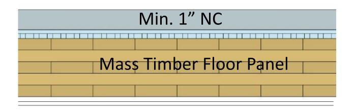
Min. 1" thick NC protection required on mass timber floors in IV-A and IV-B. Not required in IV-C
