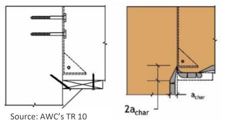
2. Engineering analysis that demonstrates that the temperature rise at any portion of the connection is limited to an average temperature rise of 250° F (139° C), and a maximum temperature rise of 325° F (181° C), for a time corresponding to the required fire resistance rating of the structural element being connected. For the purposes of this analysis, the connection includes connectors, fasteners, and portions of wood members included in the structural design of the connection.
