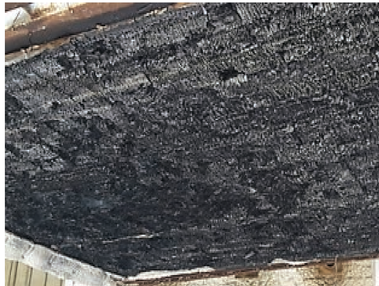
E119 test, CLT floor after 2hrs, with no char fall-off
