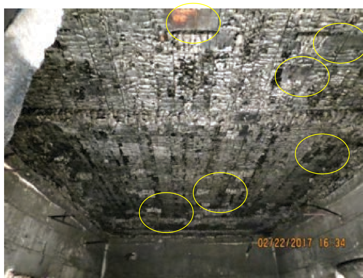
E119 test, CLT floor after 2hrs, with char fall-off
