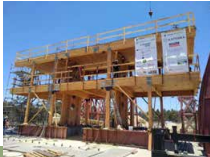
Mass Timber Shake Table Test at UCSD
