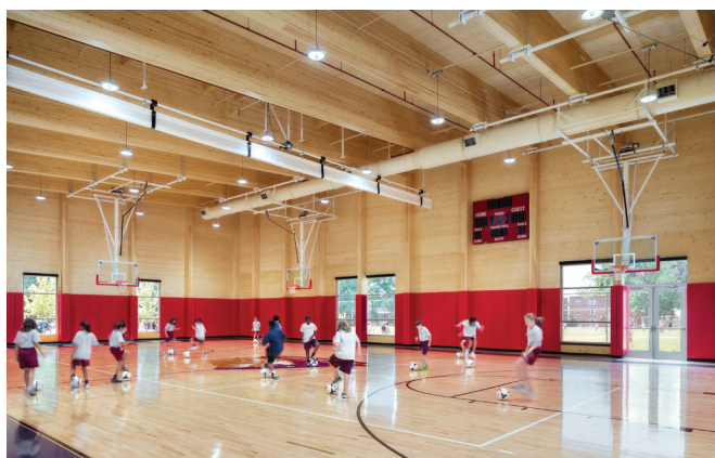
Safety padding on the lower portion of gym walls at Washington Latin Public Charter School also protects from damage.
