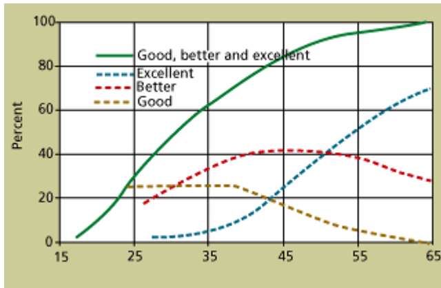
FIGURE 2: PERCENT POPULATION PERCEIVING A FLOOR TO BE GOOD TO EXCELLENT VS. FLOOR PERFORMANCE
