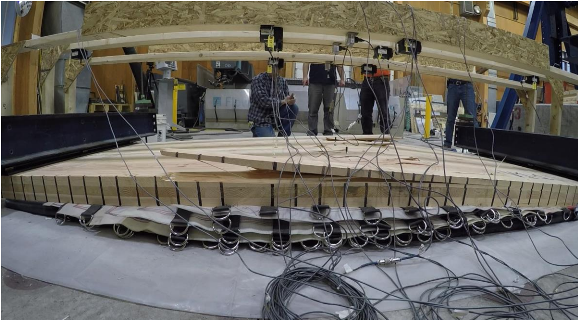
Figure 3-1. UMaine Test Apparatus with CLT Panel at Conclusion of Test.
