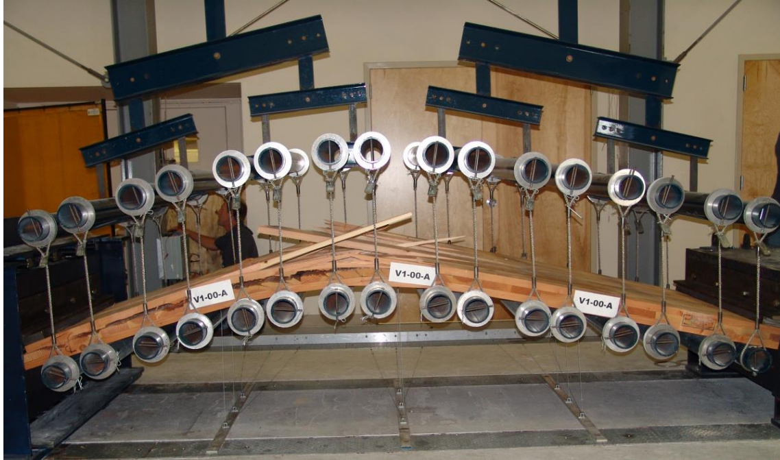
Figure 4-1. AFCEC Test Apparatus with CLT Panel at Conclusion of Test.
