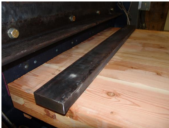
(a) 5% F_c^* – no evidence of panel edge failure.
