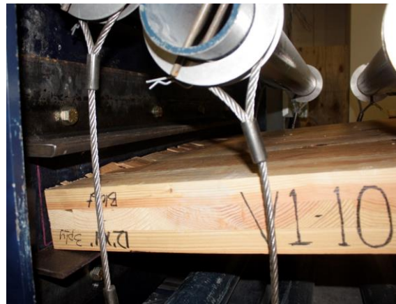
(b) 10% F_c^* – failure at top fibers due to rotational constraint provided by test apparatus.
