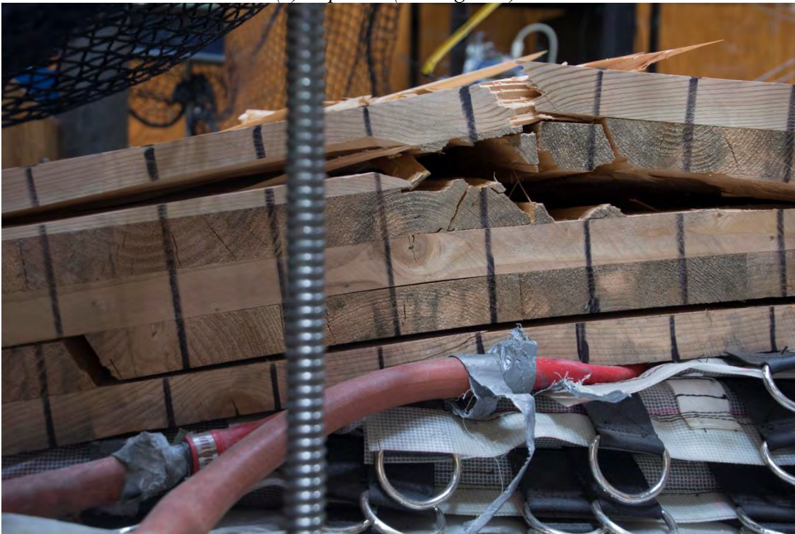
(b) Detail view (looking west). (Note slip between individual CLT plies.)
