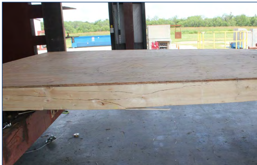
Figure 9. Test 6 Specimen Post-Test Cracking of Edge Member at Mid-Span
