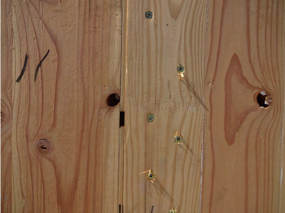
Figure 4-2. Knot Pop Out on Exposed Face of Grade V1 Test Structure Following Test 1.
