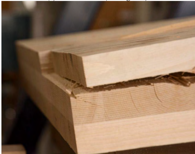
(b) Shear slip at end.
