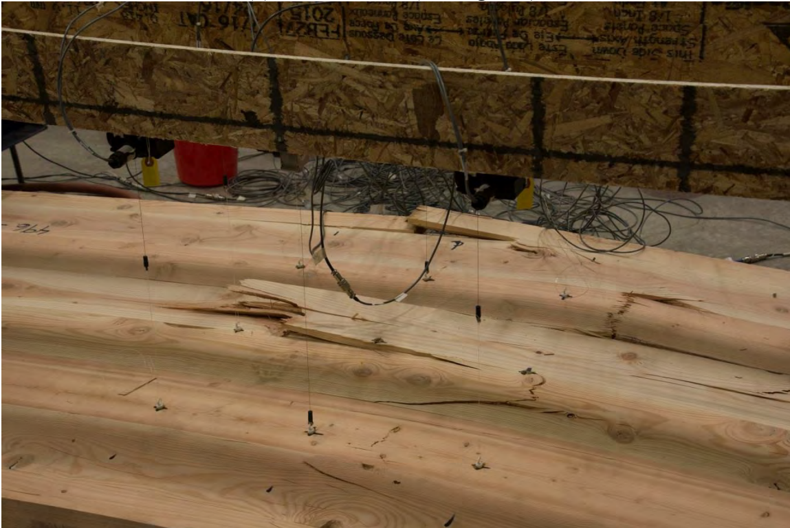
(b) Initiation of failure (looking east). (Note failure at finger joint outside middle two feet.)
