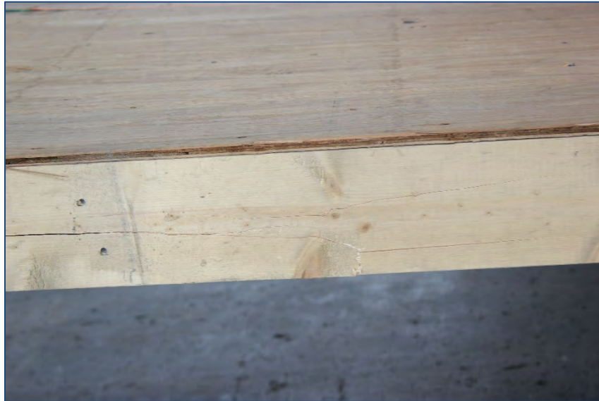
Figure 8. Test 5 Specimen Post-Test Cracking of Edge Member at Mid-Span
