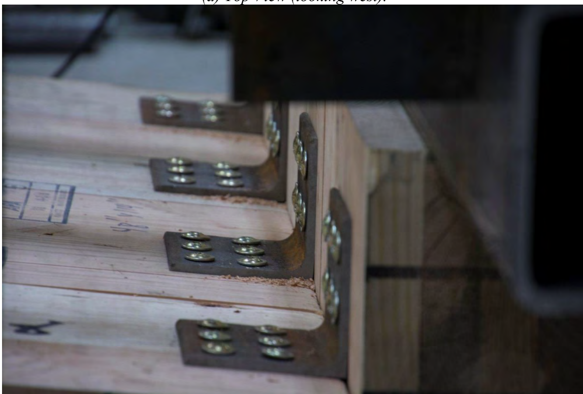
(b) Detail view – bracket deformation (looking west).
