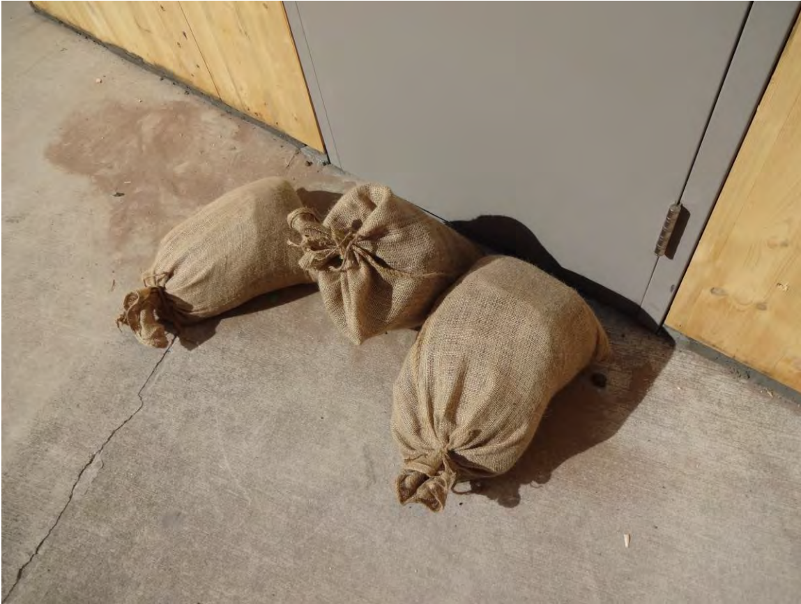
Figure 4-7. Test 2 Post-Test Photograph of Sand Bag Overturning.
