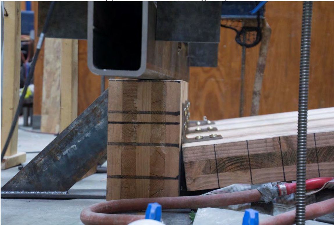
(b) Detail view – bracket deformation (looking west).
