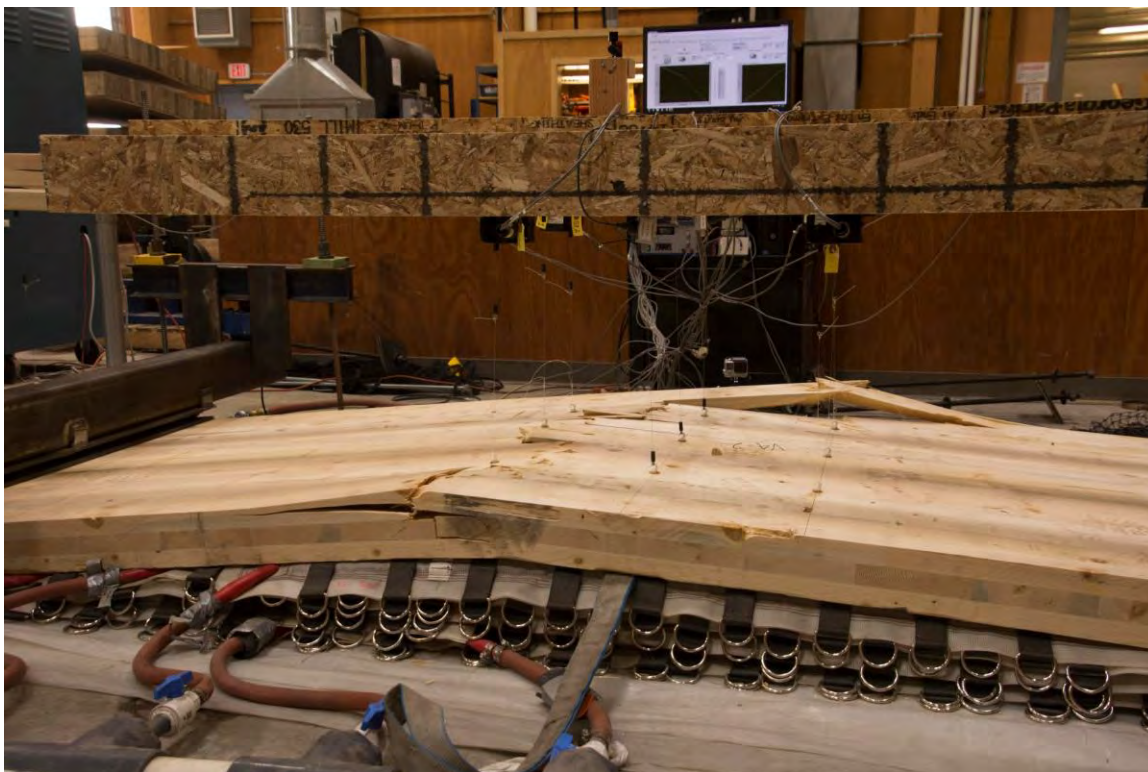
Figure A-23. 3-Ply Grade V4 CLT – Test 2 (V4-2).
