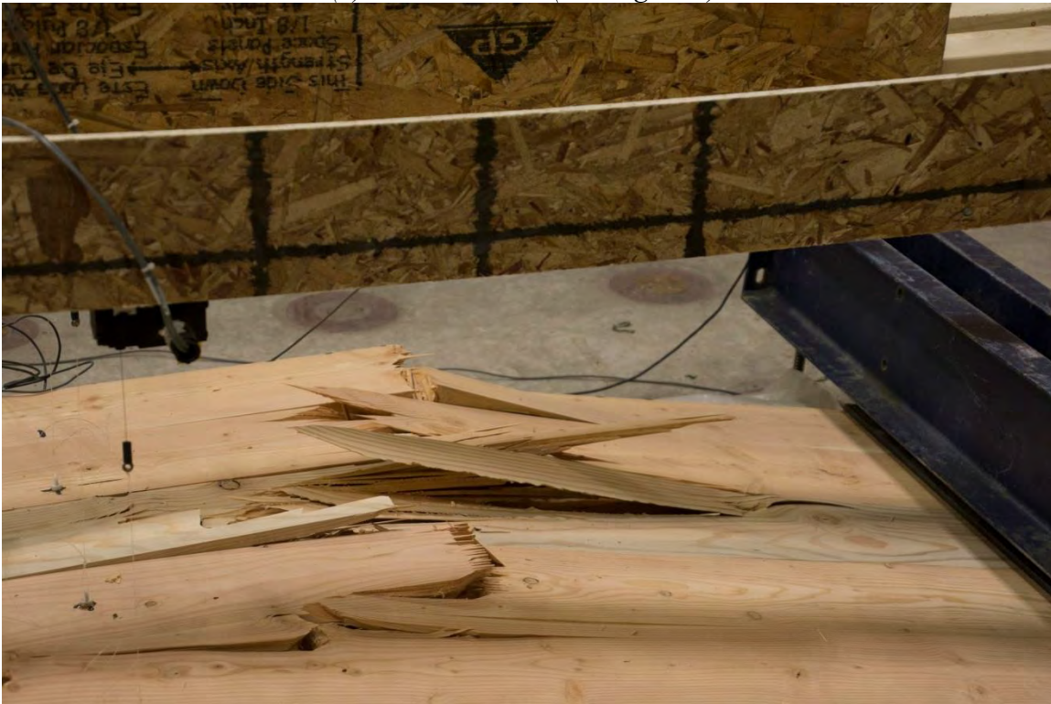
(b) Top view (looking east). (Note failure at finger joints near support, no finger joints located near panel mid-span.)
