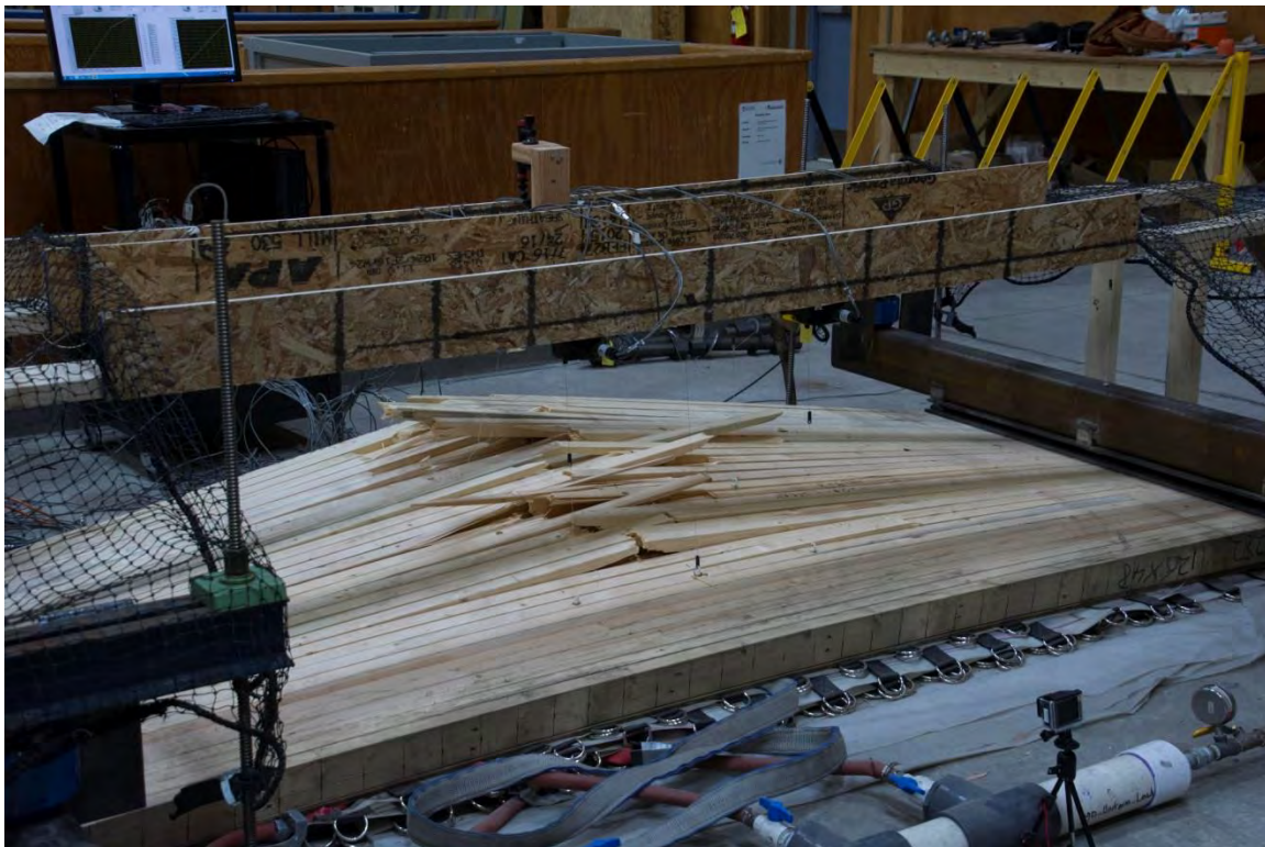
Figure 4-7. Asymmetric Flexural Failure of NLT Panel.
