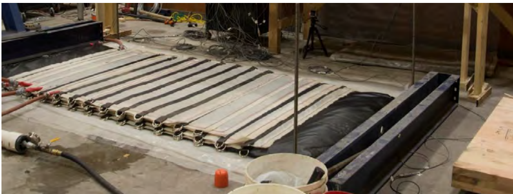
Figure 3-3. Bladders in Place Prior to Panel Placement.
