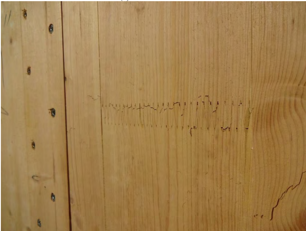
(b) Finger Joint Crack.
