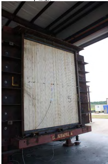
(e) Test 5: 2x6 NLT \mu_{\text{target}} = 1.00 .
