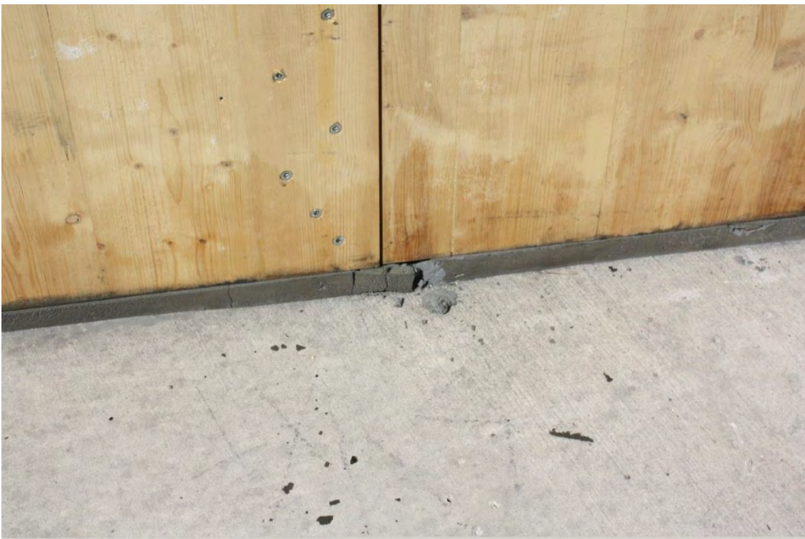
Figure 4-3. Test 1 Post-Test Photograph of Grout Breakup.
