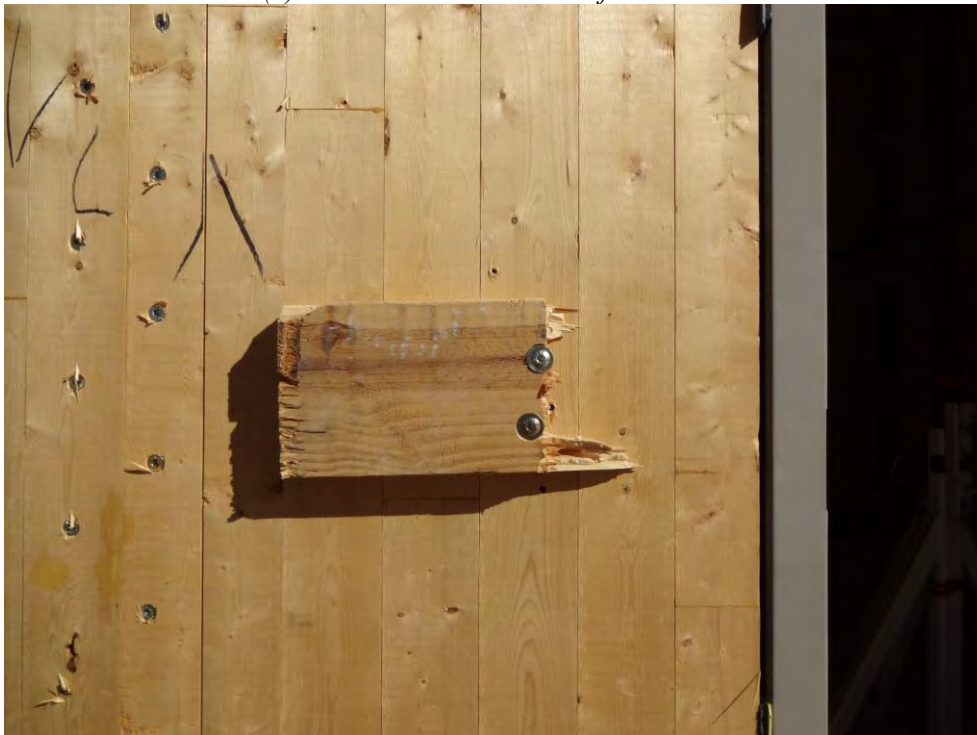
(b) 2x Restraint Rupture.
