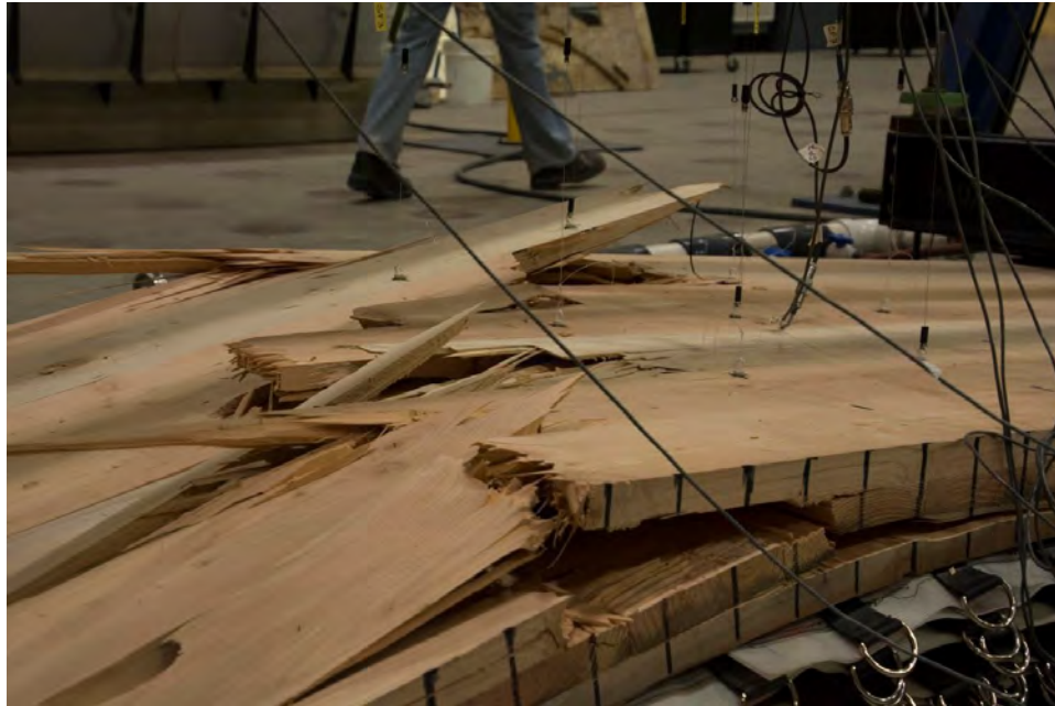
Figure 3-10. Photo of Typical 3-ply CLT Panel at End of Test.
