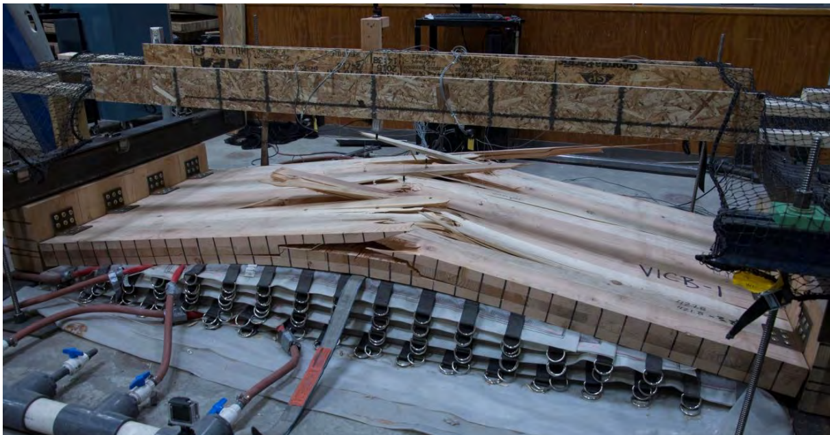
Figure 2-1. UMaine Test Apparatus with CLT Panel at Conclusion of Test.
