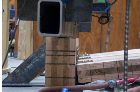
(b) Bracket Deformation.
