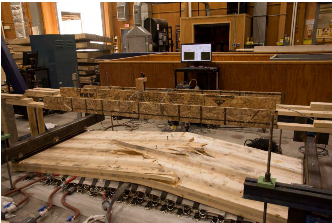
Figure A-22. 3-Ply Grade V4 CLT – Test 1 (V4-1).
