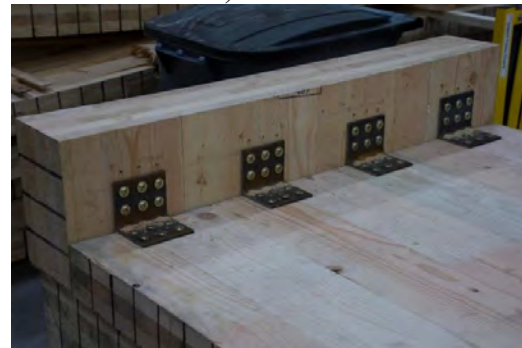
(b) L4x4x1/4 Bracket (4 bracket test shown).
