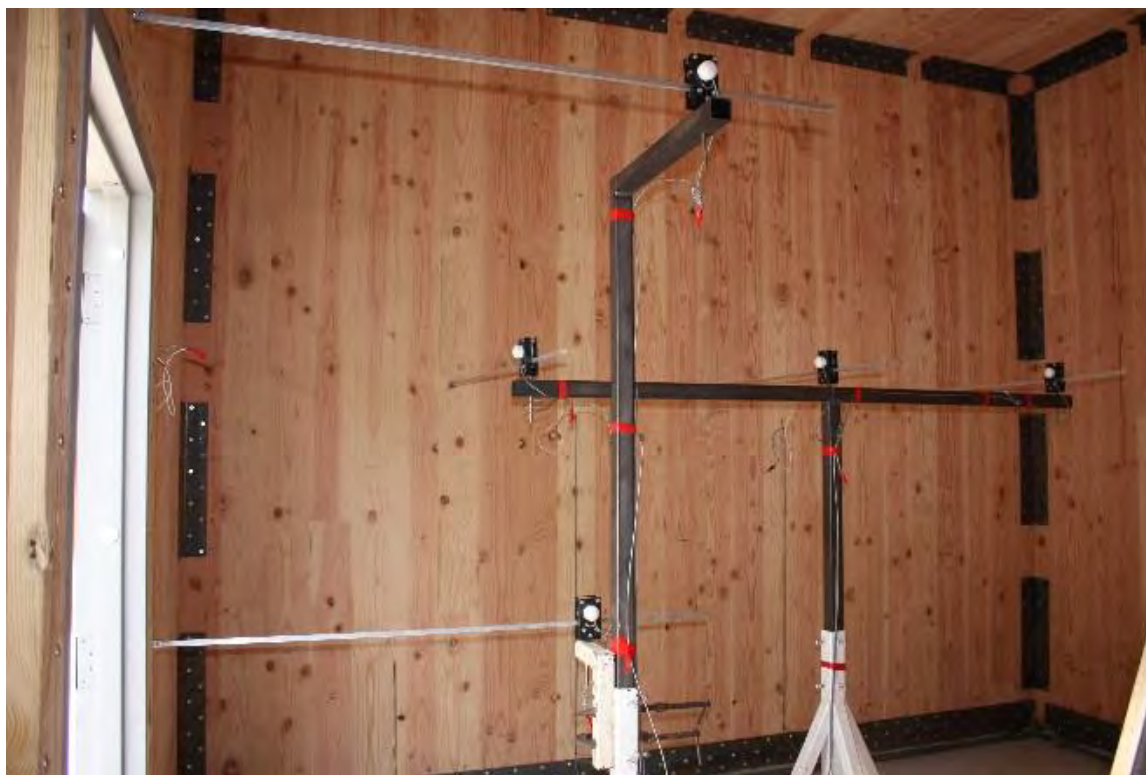
Figure 3-18. Rack and Wheel Displacement Gages with Support Stands.
