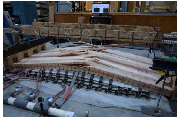
(b) Flexural Failure Associated w/ L4x4 Brackets.
