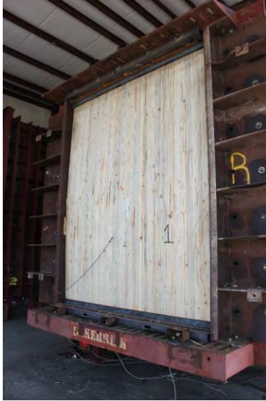
(a) Test 2: 2x4 NLT \mu_{\text{target}} = 0.75 .
