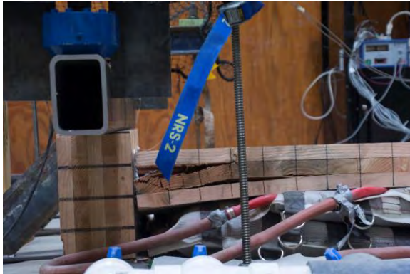
(a) Shear Failure Associated w/ SST Brackets.
