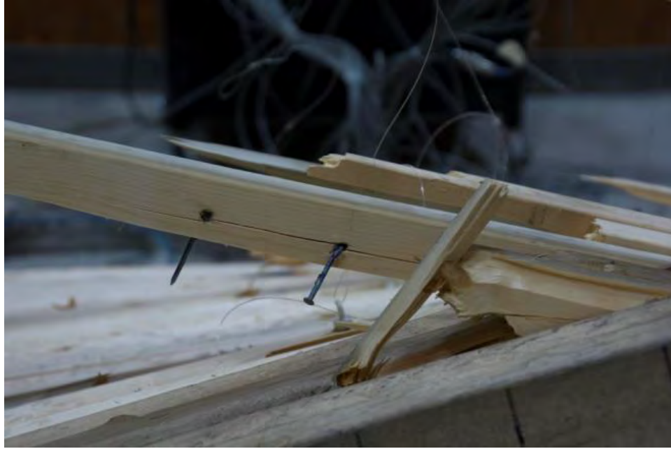
Figure 4-8. Details of NLT Panel Failure.
