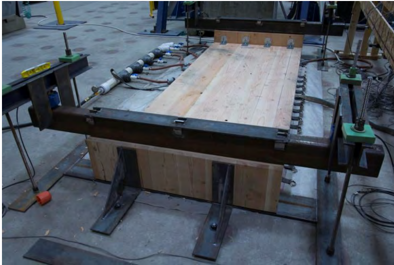
Figure 3-6. “Semi-Rigid” Test Setup Configuration.
