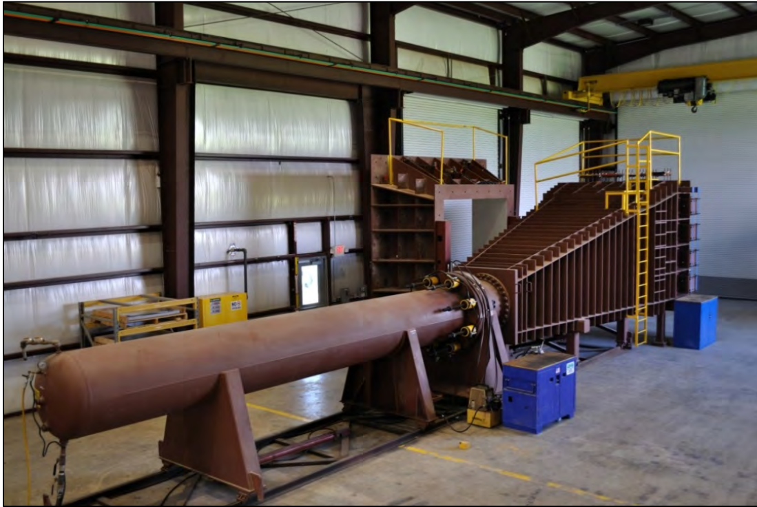
Figure 4. BakerRisk Shock Tube
