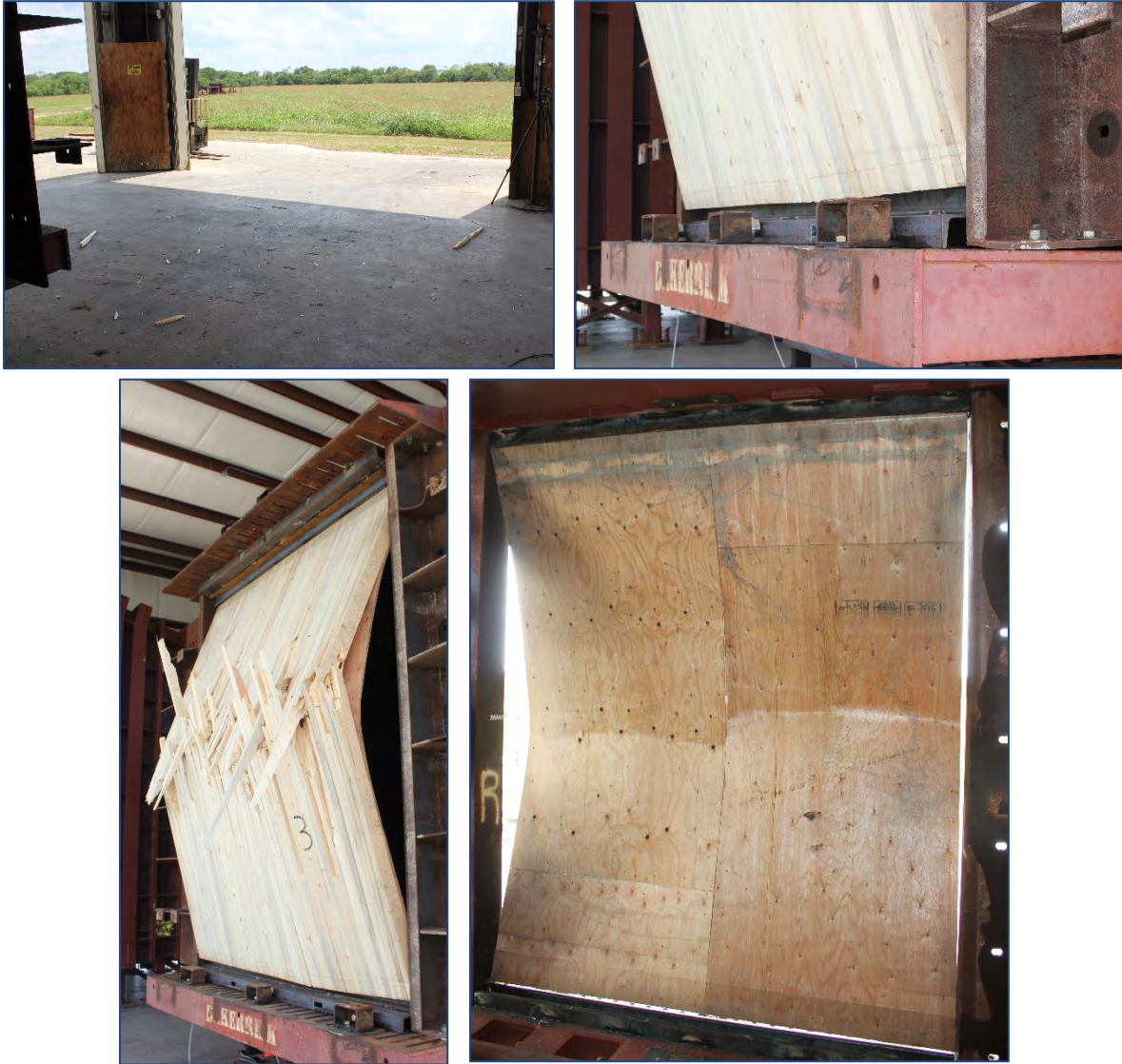
Figure 7. Test 3 Debris Field and Support Disengagement (Top) and Damage Views (Bottom)
