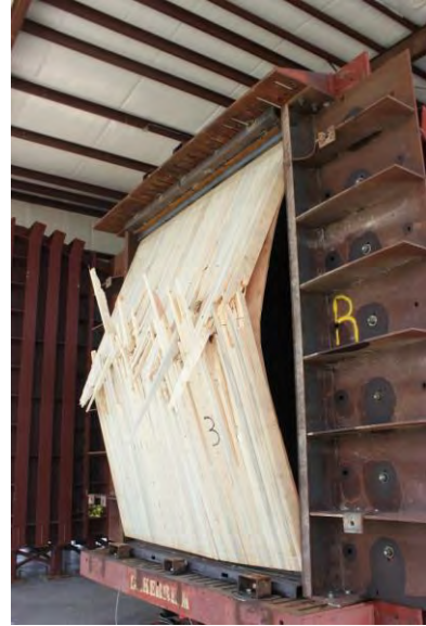
(c) Test 3: 2x4 NLT \mu_{\text{target}} = 1.25 .
