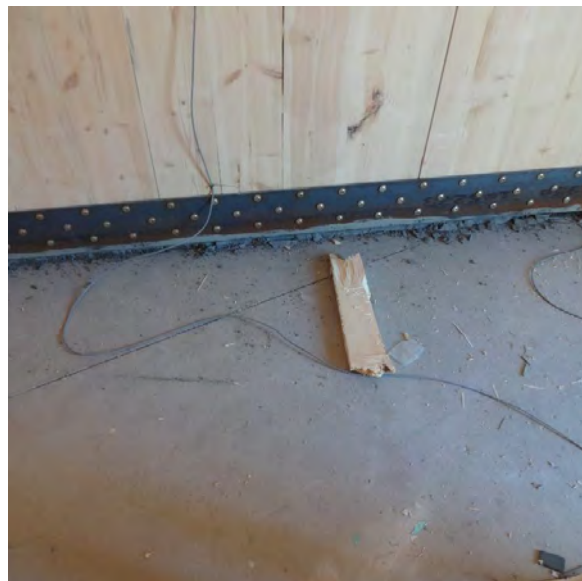
(b) Grade V4 Test Structure – Board Delamination.
