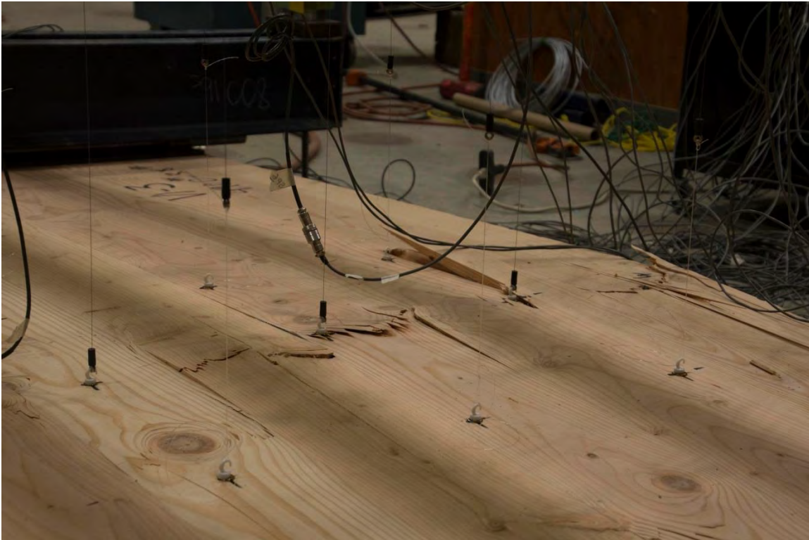
Figure 3-9. Connection of String Potentiometers to Panels.
