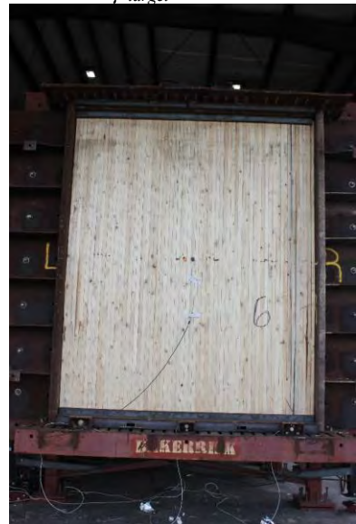
(f) Test 6: 2x6 NLT \mu_{\text{target}} = 1.25 .
