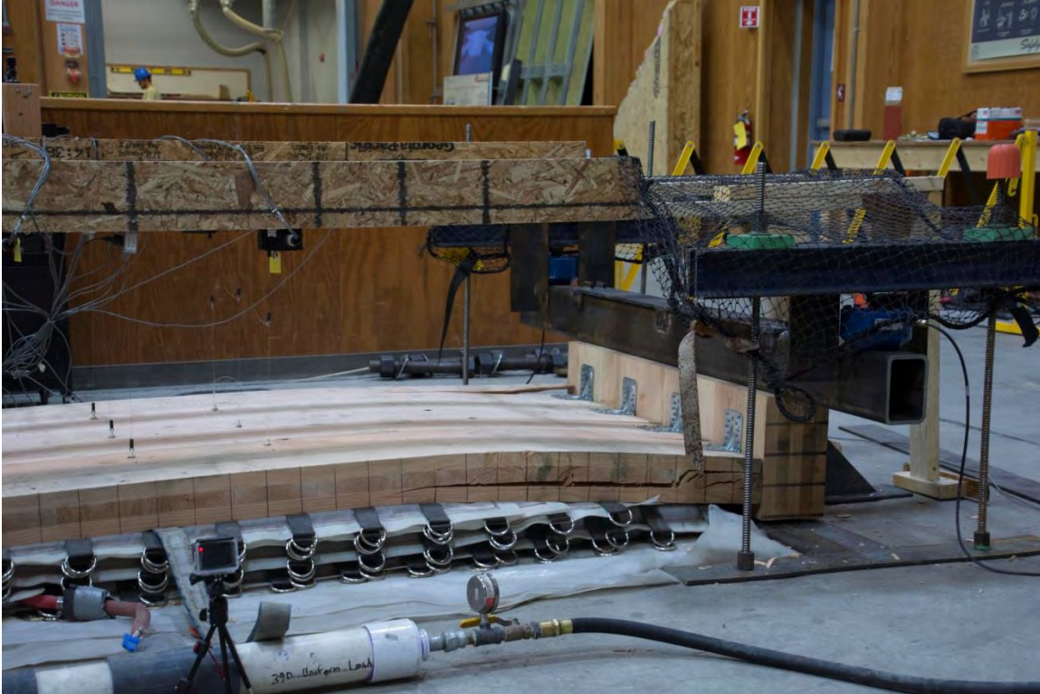
(a) Initial shear failure (looking west).
