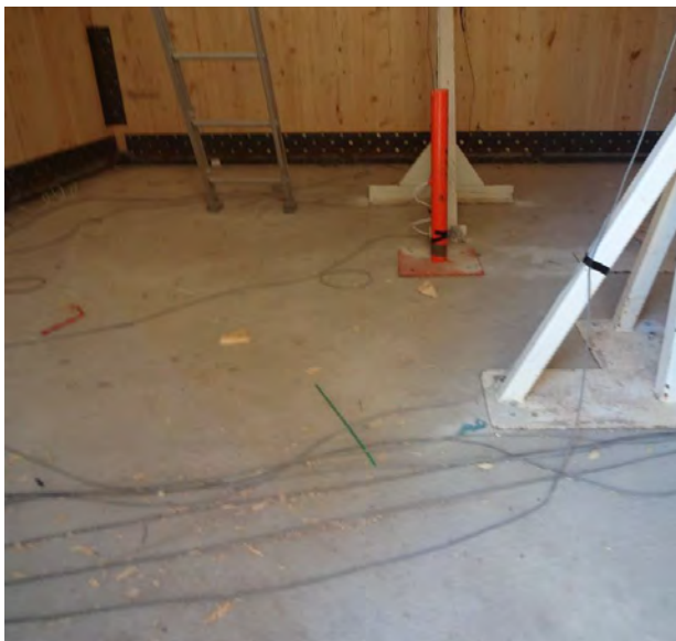
(a) Grade V4 Test Structure – Many Small Pieces of CLT Panel Debris.
