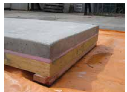
Composite floor panel used for testing Project Name: UBC Earth Sciences Building Photo credit: Equilibrium
