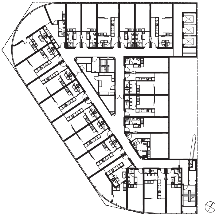
▲ Figure 2.1.2: A typical hotel floor plan (Level 10) for the upper portion of 55 Southbank. Solid walls are CLT panels, as is the base flooring. The new steel lift core, constructed for the addition, is at upper right. © Bates Smart Architects
