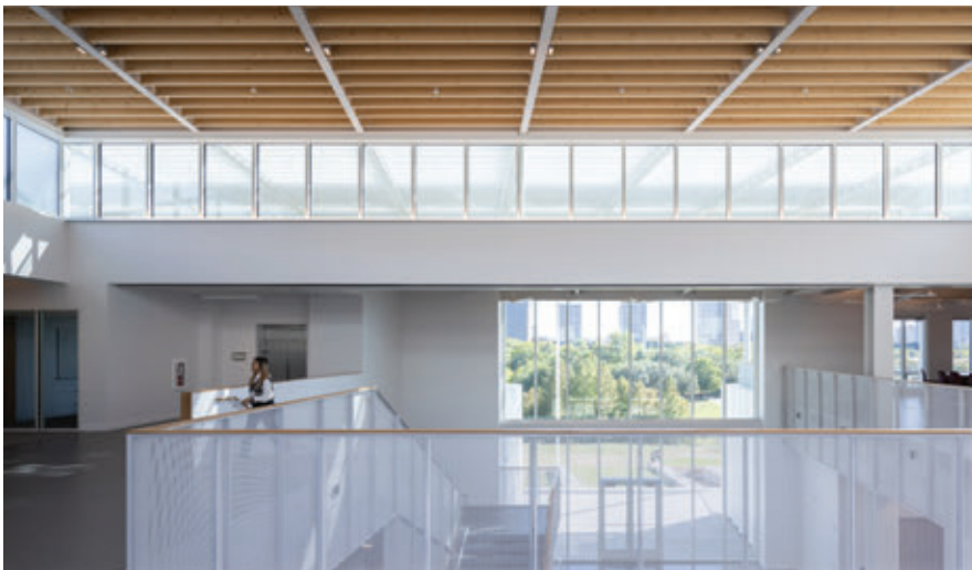
▲ Figure 2.4.3: The building interior features exposed timber and steel structure, a double-height atrium, and clerestory windows. © Kevin Daly Architects, photo by Iwan Baan
