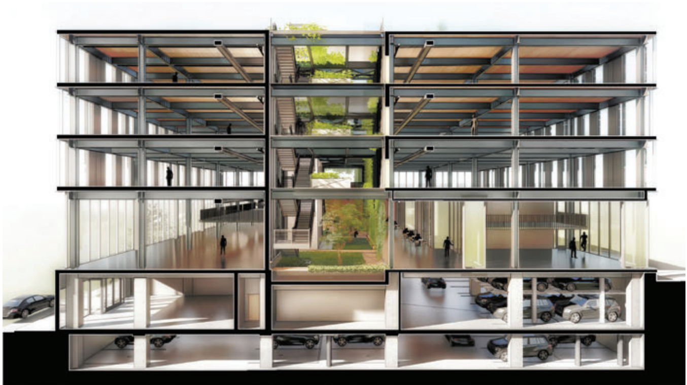
▲ Figure 2.2.3: Section perspective of 843 North Spring Street. Original concrete commercial building and parking structure is topped by a double-height space framed in steel. An open-air courtyard runs through the center, and is filled with greenery. The top three floors are framed in steel and floored in CLT. © LEVER Architecture
