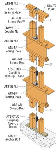
**Figure 6. Typical continuous holdown assembly**
