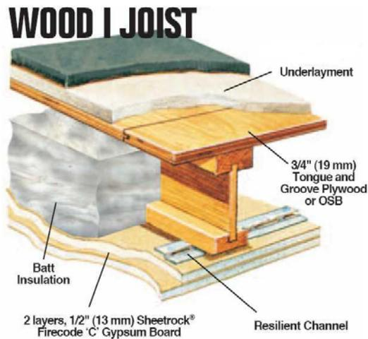
**Figure 3. Typical floor assembly**
