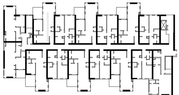
Figure 2. Typical residential building plan with central corridor (Bold walls represent shear walls)
