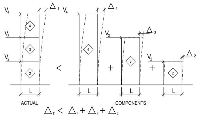
Figure 9. Assumed maximum multi-story shear wall deformation at the roof level
