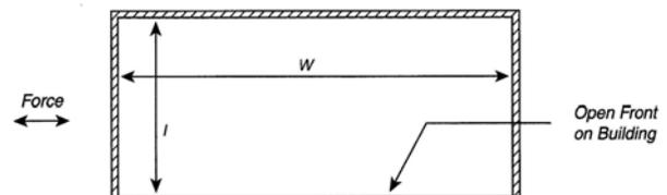
**Figure 4. Open-front Diaphragm**
