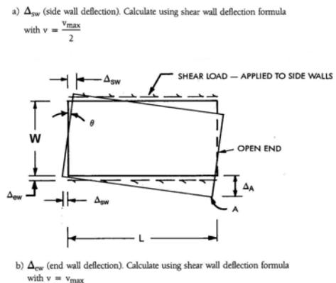
**Figure 5. Open-front Diaphragm Deflection**
