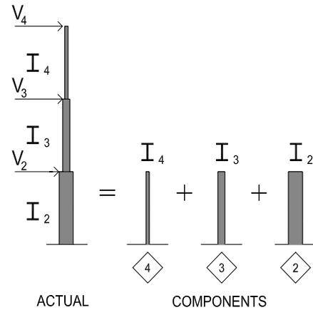
Figure 7. “Stacked” column shear wall
